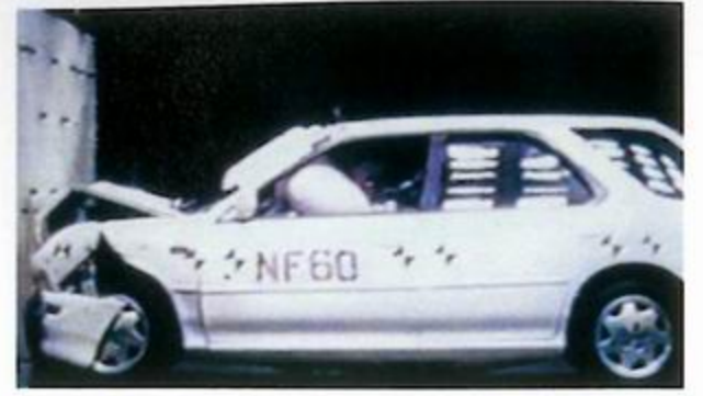
THE FRONT CRUMPLE ZONE AND THE STEERING COLUMN ARE DESIGNED TO ABSORB IMPACT ENERGY IN A FRONTAL COLLISION.
